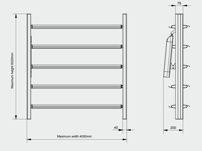
The blades and guide rails in the **Sunbreaker** system are made from |extruded aluminium.
