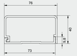
Type A blades are designed for horizontal surfaces (roofing, skylights). Owing to the special shape of the blade when in the closed position, it provides protection from rain.
